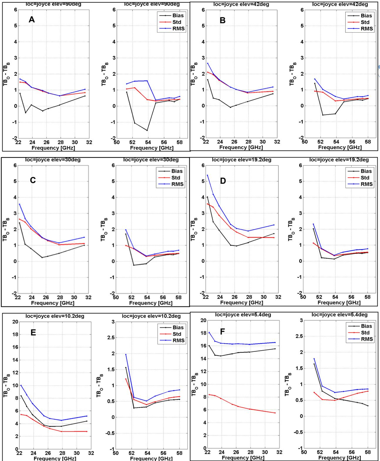
**Figure 3:** Statistics of the differences between measured TB and TB simulated with RTTOV-gb from AROME profiles for JOYCE in clear-sky conditions. Biases are shown with black lines, standard deviations with red lines and RMS with blue lines. Panels A, B, C, D, E, and F refer respectively to 90, 42, 30, 19.2, 10.2, and 5.4° elevation angle.
