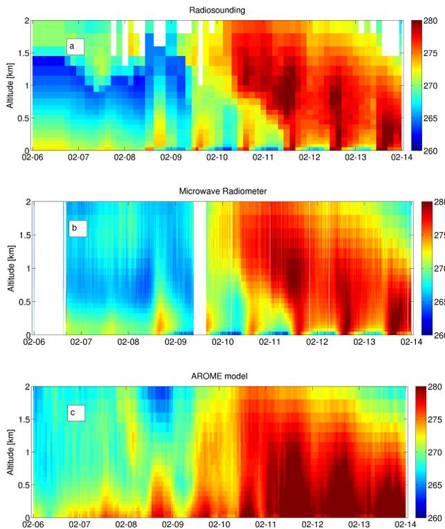
**Figure 6:** Time series of temperature profiles during IOP 1 from (a) radiosounding, (b) Microwave Radiometer, (c) AROME
