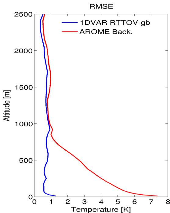
**Figure 7:** RMSE of temperature profiles with respect to radiosondes: MWR retrievals in blue, AROME 1-h forecast in red
