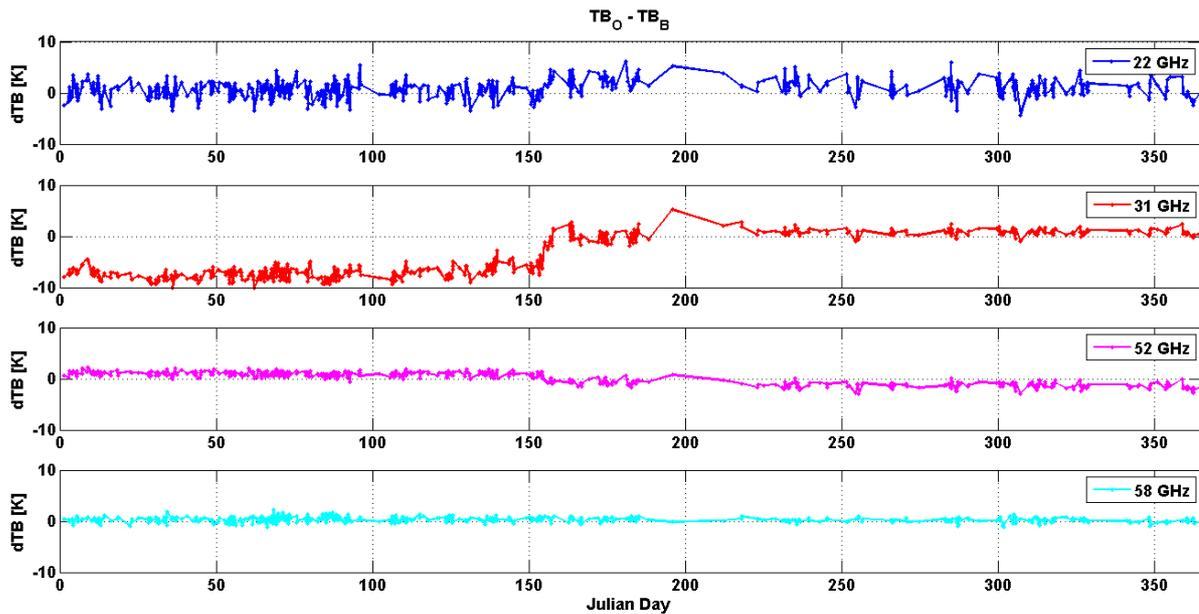
**Figure 4:** Time series of TB O-B at channel 22.24, 31.40, 52.28, and 58.0 GHz in JOYCE. The second panel from the top shows a mis-calibration of the 31 GHz channel up to Julian day 160 (3 Jun 2014).
