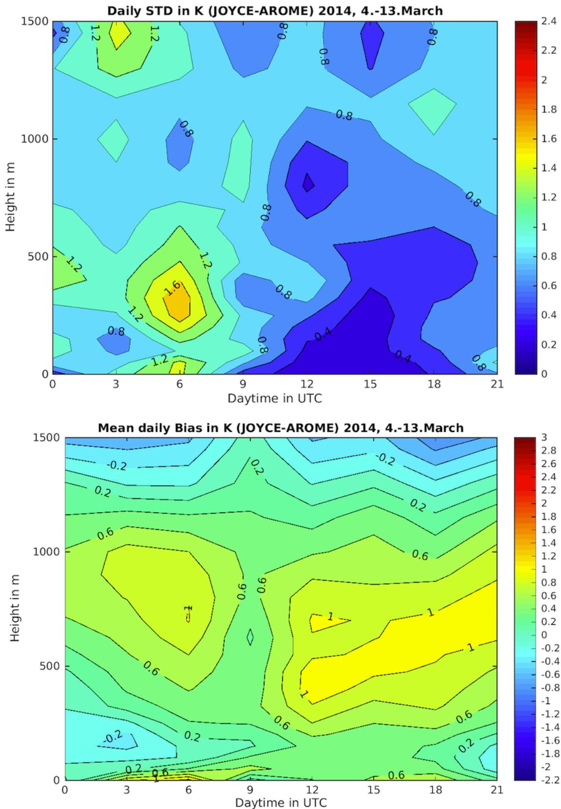
**Figure 5:** Time series temperature O-B statistics (Top: STD(MWR-AROME); Bottom BIAS(MWR-AROME)) during a 10-day period of stable high-pressure weather at JOYCE.
