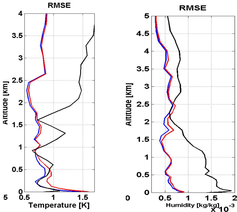
**Figure 8:** RMSE of 1D-Var retrievals against radiosondes using RTTOV-gb and Payerne MWR observations: temperature (left panel) and humidity (right panel).
