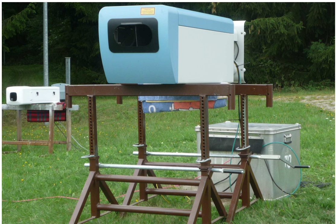
Simultaneous horizontal measurement with a CHM and a CL31 instrument. Foto by Ulrich Görsdorf (DWD, Germany).
