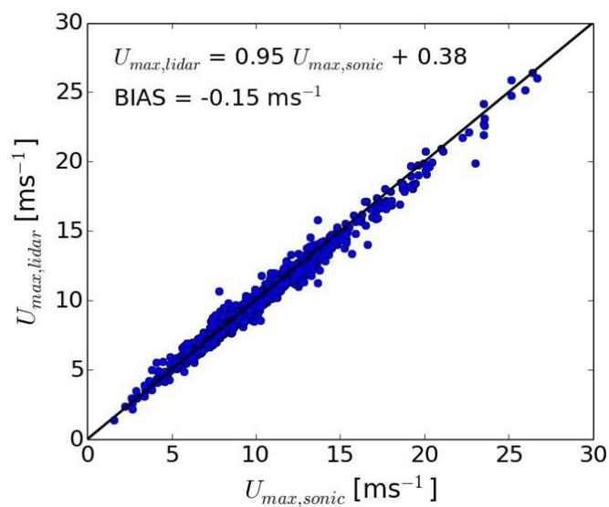
Figure 3: Comparison of wind gust speed from the lidar and the sonic anemometer at 100m level during 10.6.-8.12.2011.
