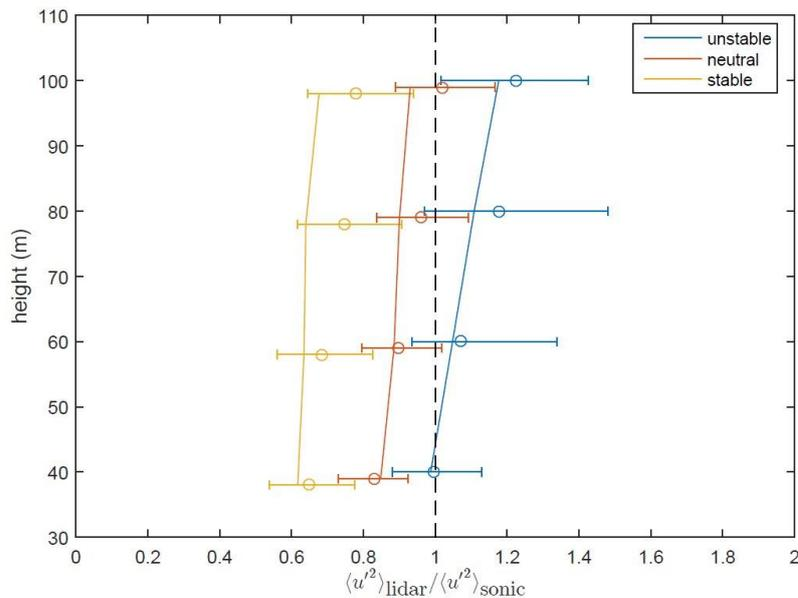
Figure 5: The ratio of the wind velocity variances from a pulsed lidar and sonic anemometer in the direction of the mean wind. Circles with error bars show the observations, vertical lines the model results (Sathe et al. 2015, their Figure 5.4b).
