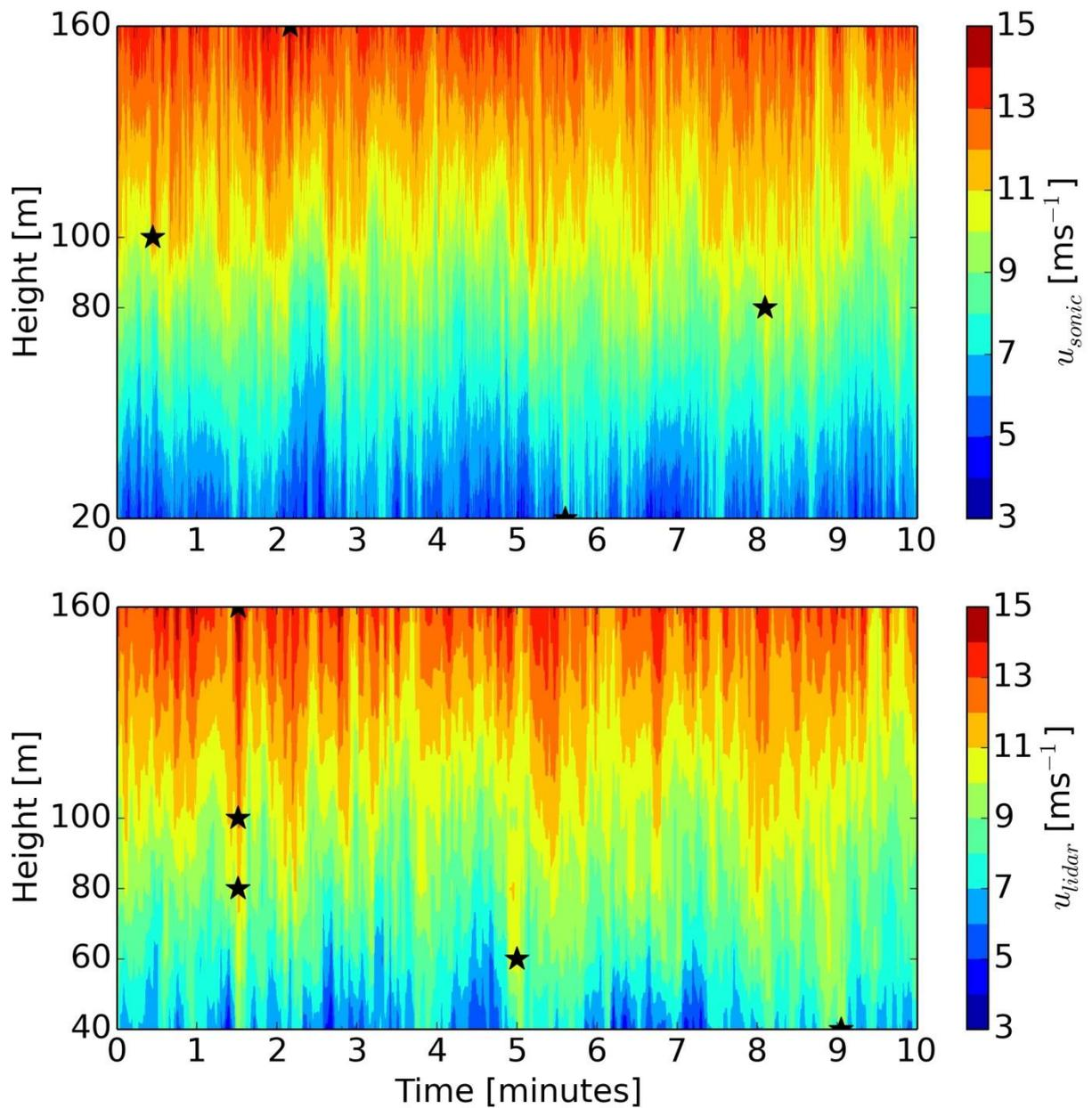
Figure 4: Example of a 10 min time-height cross-section of a sonic (top) and lidar (bottom) wind speed. The ticks on the vertical axis show the observation heights. The maximum at each observation level is presented as a black star in the plots.
