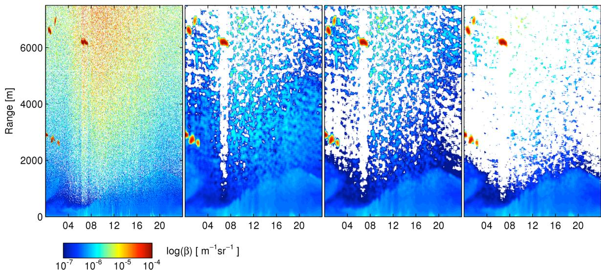
Figure 4: Observations of the CL31 ceilometer at SIRTA on 29 June 2016: (a) Range corrected attenuated backscatter, 30 s block averages of 2 s data recorded, (b) as in (a) with running average ( $\sim 25$  min,  $\sim 100$  m) applied, (c) as in (b) but including correction of instrument-related background, and (d) as in (c) but filtered for  $SNR > 0.18$ . Extracted from Figure 10, Kotthaus et al. (2016).
