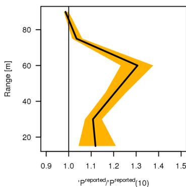
Figure 3: Median range-corrected signal ' $P^{reported}$ ' of the lowest 6 range gates (15 – 90 m) normalised by the value at the 105 m for SIRTA sensor S. Statistics calculated for all profiles observed between 11-16 UTC with ' $P^{reported} < 400 \times 10^{-8}$  a.u.' in the lowest 400 m: median (solid line) and inter-quartile range (shading).
