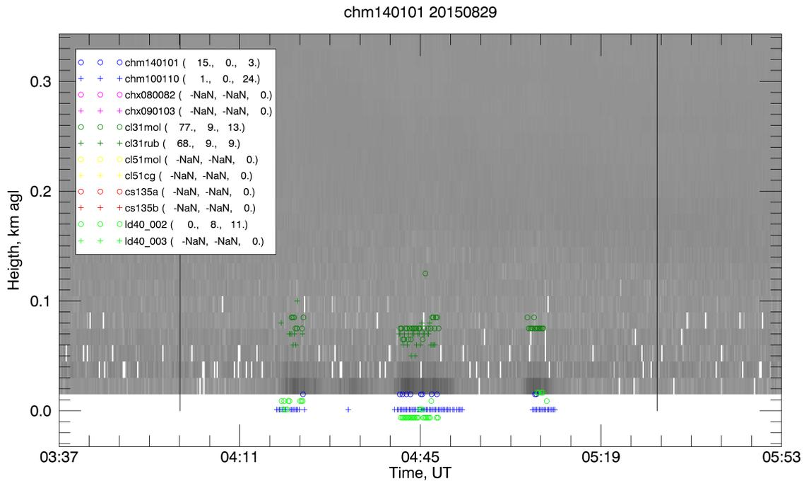
**Figure 5.** Time-height cross section of  $\beta_{att}$  (CHM15k-B) and CBH time series of all ceilometers for clear sky, the brackets in the inset contain the mean and standard deviation of CBH and the detection rate for a period marked by the vertical lines.
