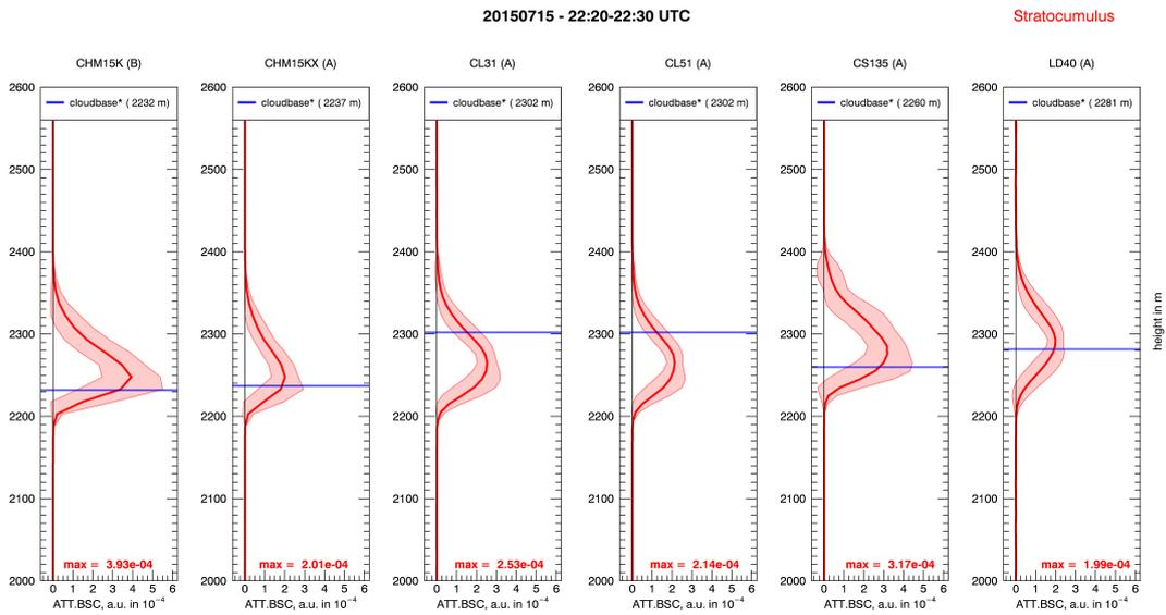
**Figure 3.** Vertical profiles of attenuated backscatter for the same day as Fig. 2. The profiles are an average over the marked period and they are normalized using an empirical factor.
