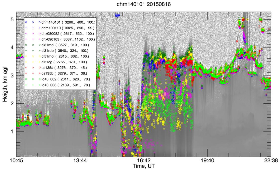
**Figure 4.** Time-height cross section of  $\beta_{att}$  (CHM15k-B) and CBH time series of all ceilometers for Cumulonimbus and temporarily heavy rain, the brackets in the inset contain the mean and standard deviation of CBH and the detection rate for a period marked by the vertical lines.
