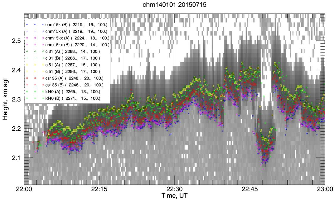
**Figure 2.** Time-height cross section of  $\beta_{att}$  (CHM15k-B) and CBH time series of all ceilometers for Stratocumulus, the brackets in the inset contain the mean and standard deviation of CBH and the detection rate for a period marked by the vertical lines.
